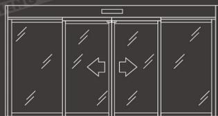
The whole evacuation system of Japan is adopted. Under normal conditions, the middle two doors automatically shift. In case of emergency, the middle two doors translation on both sides, then four doors can be all flat open, achieve full space through. Light automatic switch system can be configured.
